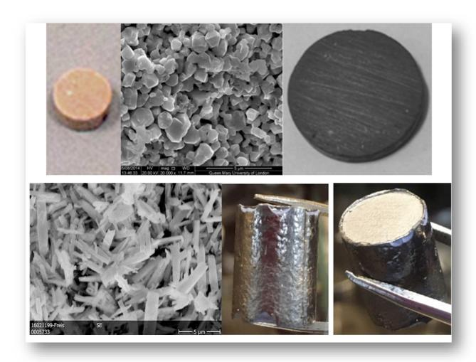
Cerium and neodymium oxide simulants were used for americium oxides in previous research. The raw material is shown in B and D and sintered discs are shown in A, C and E, Credit: E. J. Watkinson et al., 2017,
